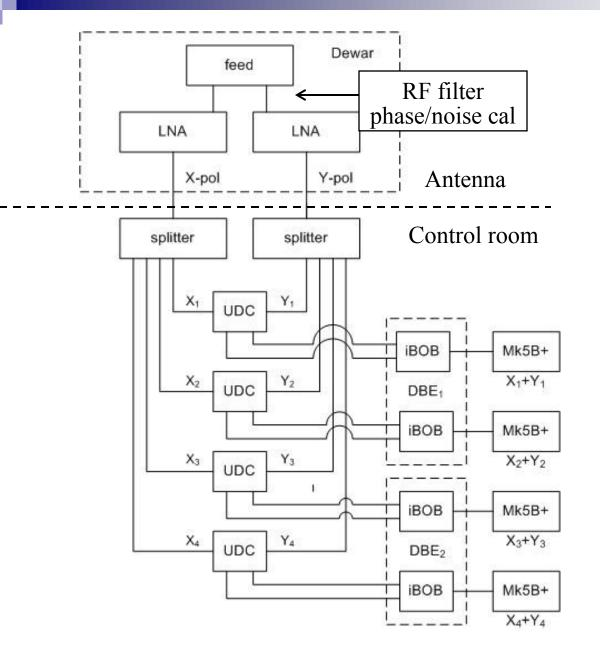
Feed and LNAs cooled to ~20K Both senses of linear polarization used
